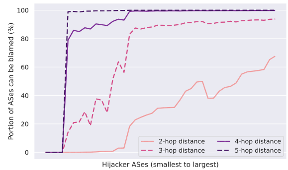
Figure 4: The portion of ASes that can be blamed as the hijack perpetrators with varying attacker ASes and their distances from the victim to be blamed.
